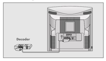
Connect the »AV1« socket on the television set and the corresponding socket on the decoder using a EURO-AV cable.
